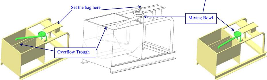
The two halves of the tank are separated in the middle by a "trough". The unmixed balls of bentonite can be allowed to wash into the trough by simply overflowing the tank on either side and thereby recirculating the unmixed material through the centrifugal pump. The 3way valves in the machine's plumbing will allow the centrifugal pump to suck out of the overflow trough or out of either tank, as needed.
