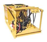
The new mixing bowl is shown to the right. As the bentonite powder travels down into the opening at the bottom of the bowl, the stream of water from the small pipe washes it away and down the horizontal pipe and in the process mixes the material with water. This is equally effective with the powder, crystal, or liquid forms of polymer.
