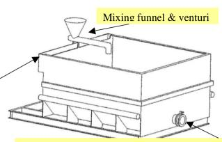
This tank drain allows the tank to be emptied quickly
