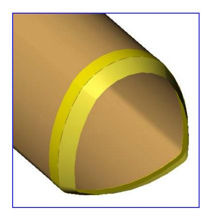
Sliplining shields are designed to
