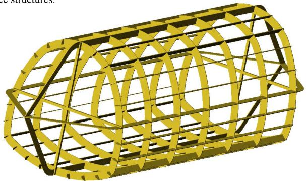
Testing mandrels are custom built to the same size and shape as the pipe used in the slipling process. The passage of the mandrel through the existing structure will ensure that the new pipe can be inserted without stoppage or delay.
