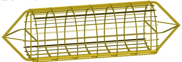
These mandrels are configured to allow the passage of the sewer stream while the mandrel is pulled in either direction. In the absence of live flow – these mandrels allow for man entry to remove obstructions.
